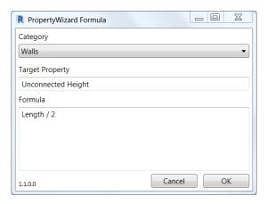
This formula sets the wall's Unconnected Height equal to half the Length of the wall.
